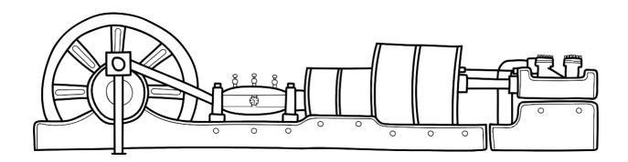
These machines used the steam from the boilers to power a water pump which you can see when you reach the other end of the engine.
