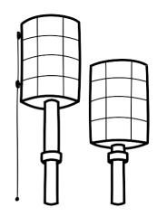
These accumulators stored pressurised water and were filled with water by the water pump on the steam pumping engine.
