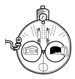
These created steam by burning coal and boiling the water. Each boiler has 2 fires and these fires were burning 24 hours a day.
